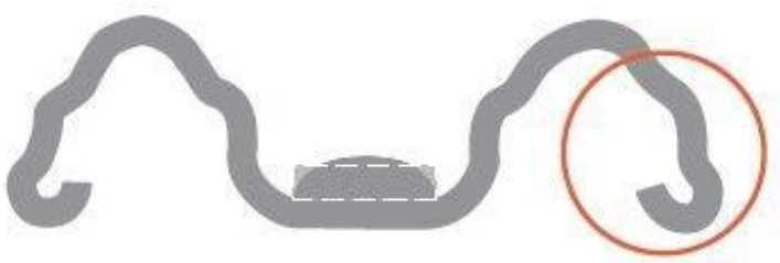
Pale cross-section and protected fixing position
